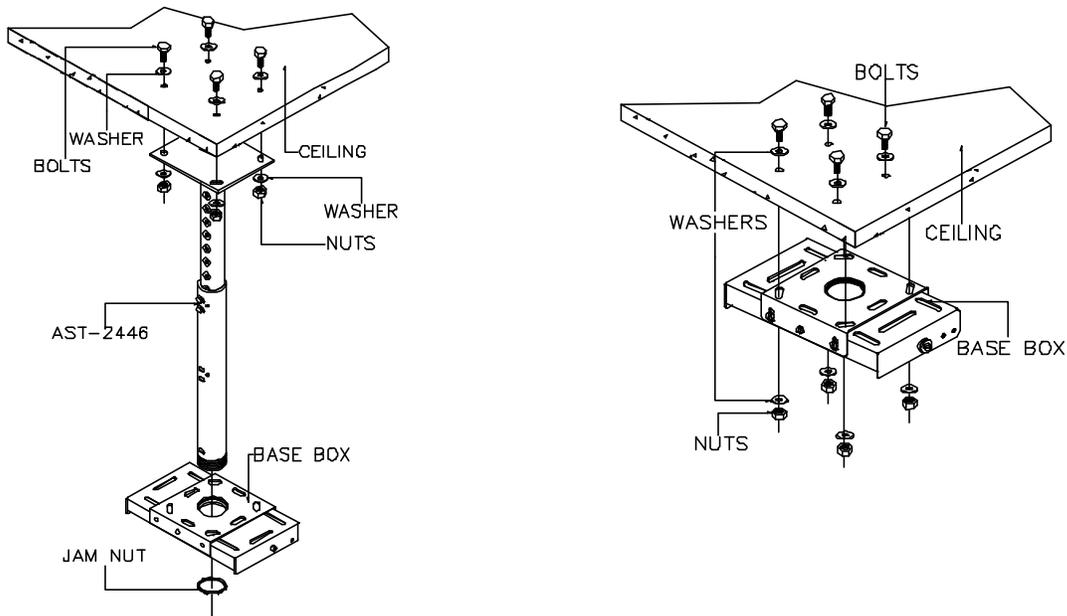
**NOTE:** If (Optional) **AST-2446** adjustable height suspension adapter is a part of the installation, securely install the adapter to the ceiling at this time. ( Refer to its installation instructions. )
